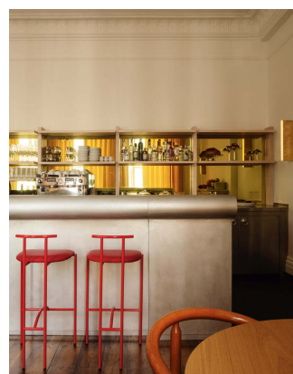
This bespoke bar designed by Daytrip for Cromwell Place Café in London is clad in naturally patinated zinc buffed to a silvery sheen – with a deep, cantilevering bullnose.
